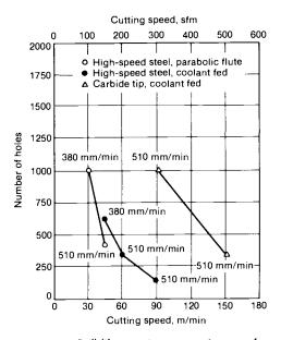
Fig. 21 Drill life at various penetratian rates for several types of drills when drilling permonent mold 390 aluminum allay. Source: Ref 2
