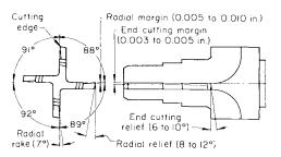
Fig. 20 Design of a finishing reamer used for reaming aluminum in automatic bar and chucking machines. Dimensions given in inches
