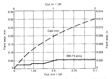
Fig. 17 Typical tool wear when broaching with a carbide cutting tool at 45 m/min (150 sfm). Source: Ref 2
