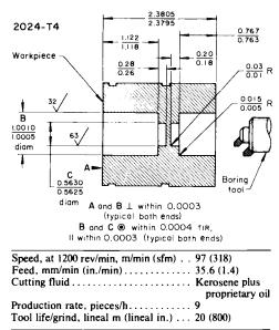
Fig. 15 Rough and finish boring of a heat-treated aluminum alloy forging. Dimensions in figure given in inches
