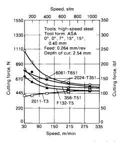
Fig. 5 The effect of speed on cutting force for five oluminum olloys
