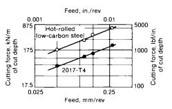
Fig. 2 The effect of feed on cutting force for low-carbon steel and aluminum alloy 2017-T4 with comparable mechanical properties
