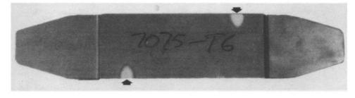
Fig. 9 Attachment tee made of 7075-T6 aluminum with the soft spot area having a hardness of 73 to 83 HRB compared to 90 HRB for the rest of the structure. Courtesy of McDonnell Douglas Canada, Ltd.
