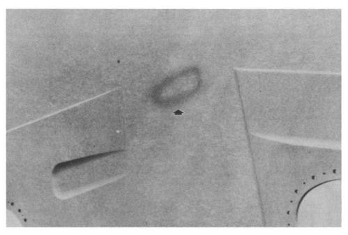
Fig. 8 Milling defect associated with the NC machining af 7075-T7651 aluminum plate with a 75 mm (3 in.) diam milling cutter. Courtesy of McDonnell Douglas Canada, Ltd.
