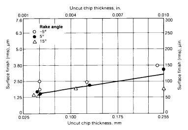
Fig. 18 Surface finish at various depths of cut when broaching 390 aluminum alloy of 100 HB at 45 m/min (150 sfm) with a carbide tool. Although the rake angle varied, the shear angle of the tool was 0° in all three cases. Source: Ref 2
