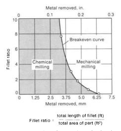
Fig. 38 Breakeven between chemical and mechanical milling. Choice between them depends on fillet ratio and depth of cut.
