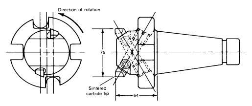
Fig. 24 Special two-cut tooth end mill with sintered carbide cutters. Dimensions given in millimeters. Source: Ref 4
