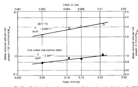
Fig. 3 The effect of feed on metal removal rate per net power for low-carbon steel and aluminum alloy 2017-T4 with comporable mechanical properties. V/NHP, volume per net horsepower
