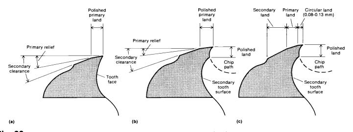
Fig. 23 Three end mill geometries designed for the cutting of aluminum alloys. (a) Conventional milling. (b) Heavy metal removal. (c) Finishing operations. Source: Ref 1
