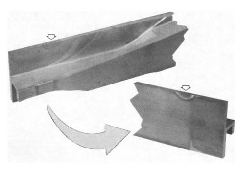
Fig. 6 Typical spar mill defect at a section change. Courtesy of McDonnell Douglas Canada, Ltd.
