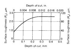
Fig. 36 Relationship between surface finish and depth of cut for the chemical milling of 7075 aluminum sheet. Source: Ref 5
