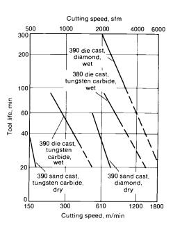
Fig. 14 Tool life curves for the dry turning of sand cast alloy 390 using carbide and diamond, the wet turning of die cast alloy 390 using carbide and diamond, and the wet turning of die cast alloy 380 using carbide. Source: Ref 2
