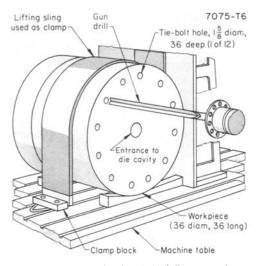
Fig. 19 Setup far deep-hale drilling an explasive farming die in a boring mill. Dimensians given in inches
