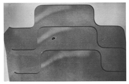
Fig. 11 Occurrence of soft spots in the same location on each of three 7075-T651 aluminum plate components. Of the 19 parts produced, 13 had a soft zone hardness of 68 to 87 HRB and conductivity of 36 to 39%. Unaffected regions of the plate had a hardness of 90 to 91 HRB and conductivity of 31 to 32%. Courtesy of McDannell Dauglas Canada, Ltd.
