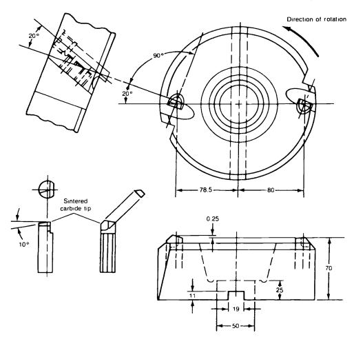
Fig. 25 Tool geometry for special two-tooth sintered carbide-tip milling cutter used to cut aluminum alloys. Dimensions given in millimeters. Source: Ref 4
