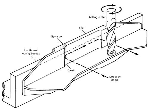
Fig. 10 Schematic of the milling cutter path in machining the attachment tee shown in Fig. 9
