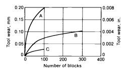
Tool wear curves for the single-tooth mill-Fig. 29 ing of alloy 390 engine blocks (wet) at 0.30 mm/rev (0.012 in./rev), A, carbide, 150 m/min (492 sfm); B, diamond, 1500 m/min (4920 sfm); C, diamond, 150 m/min (492 sfm). Source: Ref 2
