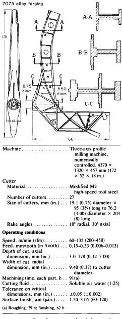
Part that was machined from a large Fig. 28 Part that was incomined willing. Dimensions in figure given in inches
