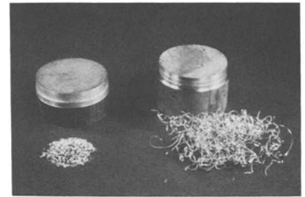
Fig. 14 Machining chips from a wrought aluminum alloy (right) and from a P/M aluminum alloy (left)
