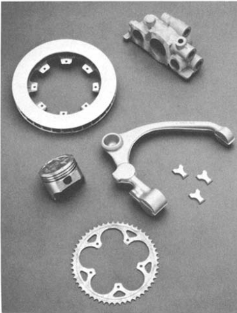
Fig. 2 Discontinuous silicon carbide/aluminum castings. Pictured are a sand cast automotive disk brake rotor and upper control arm, a permanent mold cast piston, a high-pressure die cast bicycle sprocket, an investment cast aircraft hydraulic manifold, and three investment cast engine cylinder inserts. Courtesy of Dural Aluminum Composites Corporation
