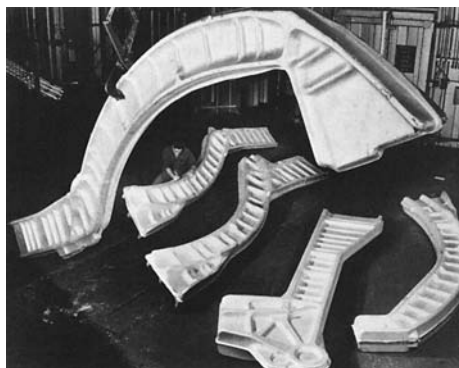
Fig. 9 Examples of very large blocker-type aluminum alloy airframe forgings
