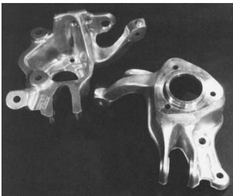
Fig. 8 Complex aluminum alloy automotive suspension components forged on a mechanical press
