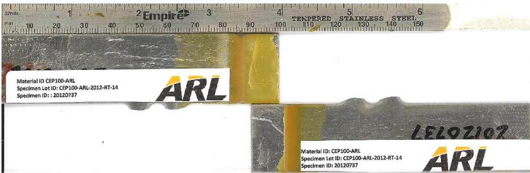
Fig. 13 CEP100 sample showing a “very good” fillet with a “very good” adhesive fill
