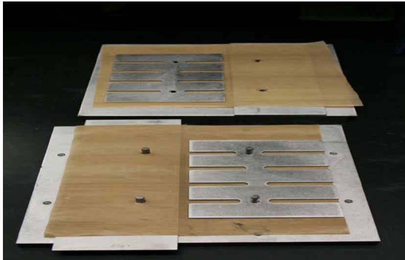
Fig. 3 Single-lap-joint tooling fixtures were used to ensure accurate joint overlap and alignment. Spacer shims controlled the bondline thickness.
