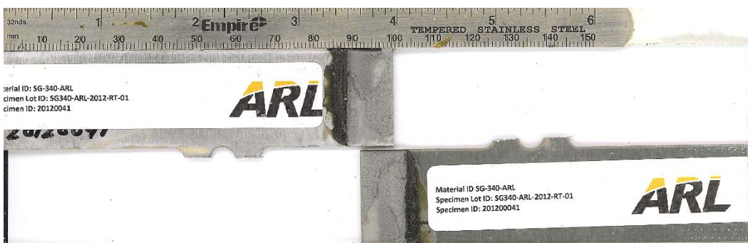
Fig. 15 SG300 sample showing a “very good” fillet with a “very good” adhesive fill
