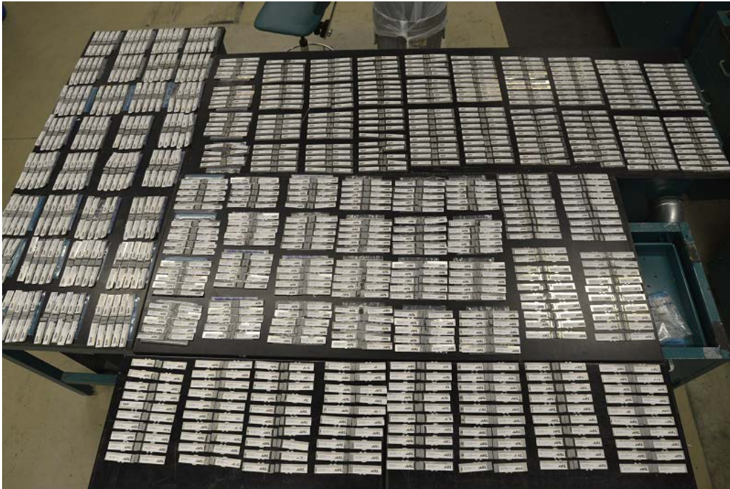
Fig. 12 Entire SG300 sample set presented for categorical assignment of mode of failure, fillet quality, and adhesive fill quality
