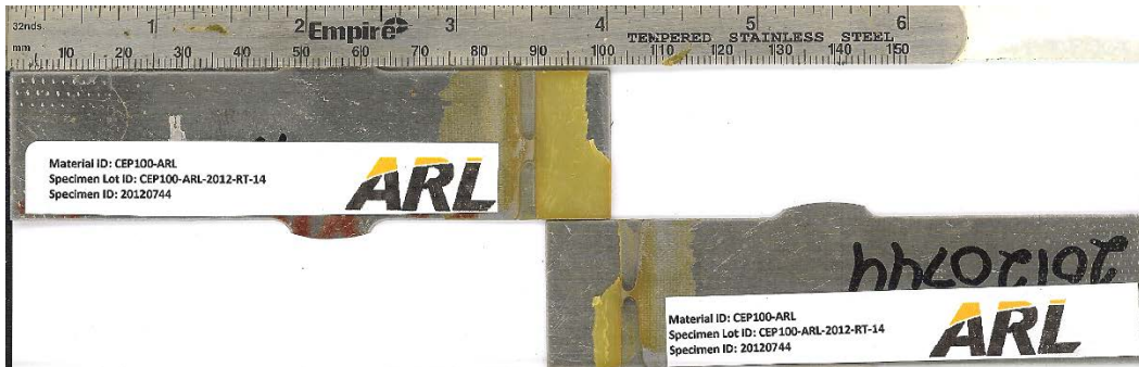
Fig. 14 CEP100 sample showing a “very poor” fillet with a “very good” adhesive fill
