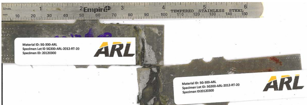
Fig. 16 SG300 sample showing a “very poor” fillet with a “very poor” adhesive fill
