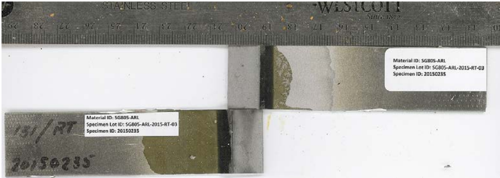
Fig. B-6 Failure surfaces for single-lap-joint with AC-131 BB surface pretreatment. MSAT ID = 20150235, substrate = 2024 T3 aluminum, and sample conditioning = RT. Mode-of-failure = MM.
