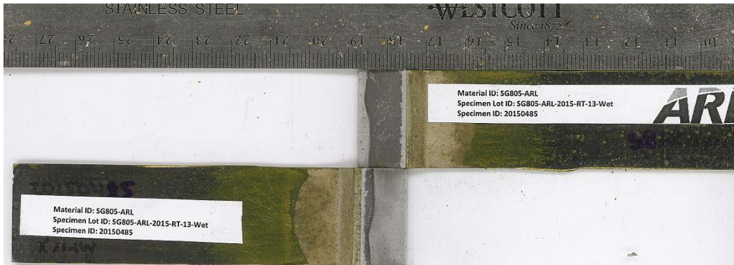
Fig. B-58 Failure surfaces for single-lap-joint with XBOND 4000DM-DR surface pretreatment. MSAT ID = 20150485, substrate = 1010 steel, and sample conditioning = H/W. Mode-of-failure = MM.
