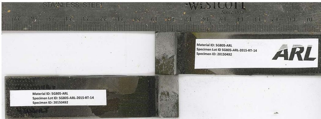
Fig. B-48 Failure surfaces for single-lap-joint with ZIRCOBOND 4200 surface pretreatment. MSAT ID = 20150492, substrate = 1010 steel, and sample conditioning = RT. Mode-of-failure = MM.
