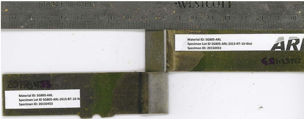
Fig. B-52 Failure surfaces for single-lap-joint with SurTec 650 surface pretreatment. MSAT ID = 20150453, substrate = 1010 steel, and sample conditioning = H/W. Mode-of-failure = MM.
