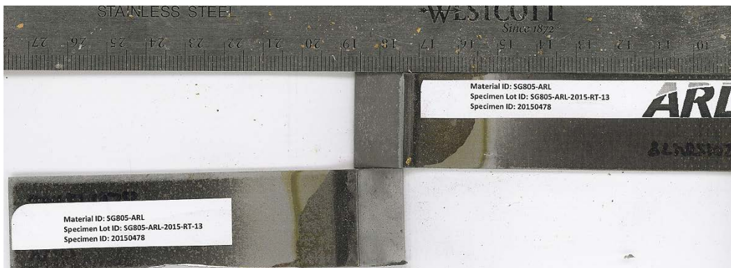
Fig. B-46 Failure surfaces for single-lap-joint with XBOND 4000DM-DR surface pretreatment. MSAT ID = 20150478, substrate = 1010 steel, and sample conditioning = RT. Mode-of-failure = MM.
