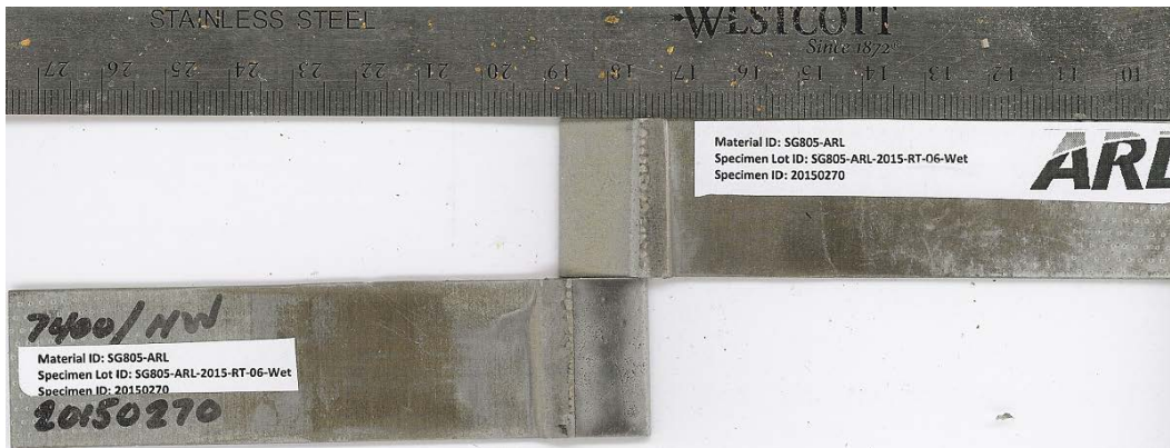
Fig. B-28 Failure surfaces for single-lap-joint with Bonderite M-NT 7400 surface pretreatment. MSAT ID = 20150270, substrate = 2024 T3 aluminum, and sample conditioning = H/W. Mode-of-failure = adhesive/ MM.
