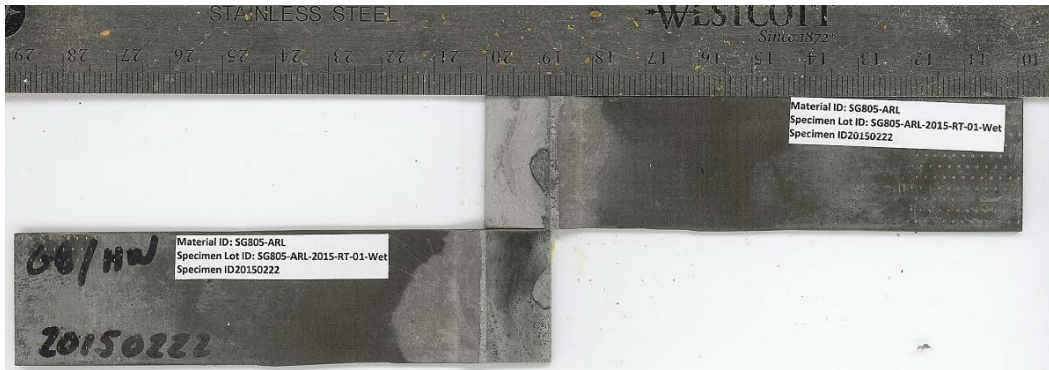
Fig. B-18 Failure surfaces for single-lap-joint with aluminum oxide grit blast surface pretreatment. MSAT ID = 20150222, substrate = 2024 T3 aluminum, and sample conditioning = H/W. Mode-of-failure = MM.
