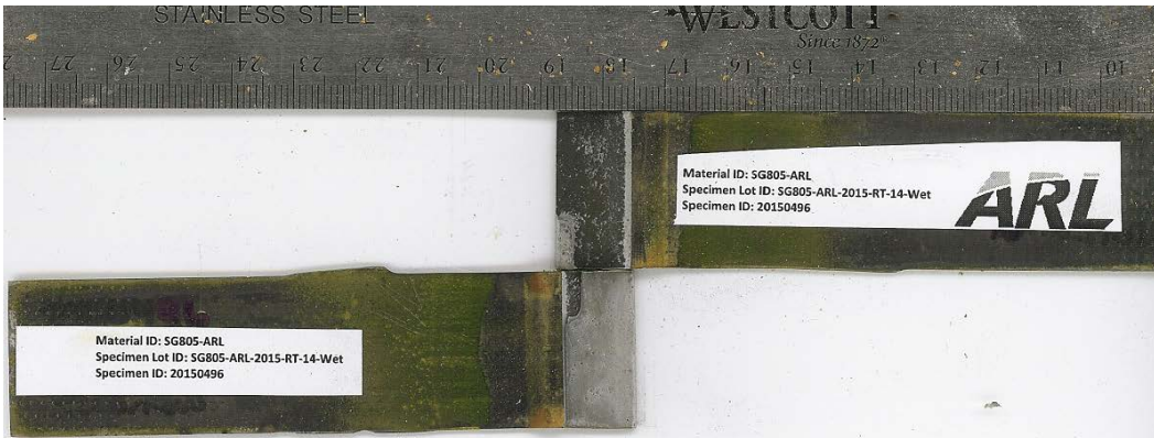
Fig. B-60 Failure surfaces for single-lap-joint with ZIRCOBOND 4200 surface pretreatment. MSAT ID = 20150496, substrate = 1010 steel, and sample conditioning = H/W. Mode-of-failure = MM.
