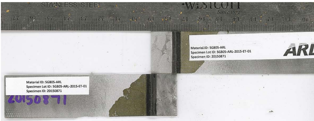
Fig. B-34 Failure surfaces for single-lap-joint with aluminum oxide grit blast surface pretreatment. MSAT ID = 20150871, substrate = 2024 T3 aluminum, and test conditions = ET. Mode-of-failure = MM.
