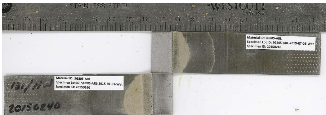
Fig. B-22 Failure surfaces for single-lap-joint with AC-131 BB surface pretreatment. MSAT ID = 20150240, substrate = 2024 T3 aluminum, and sample conditioning = H/W. Mode-of-failure = MM.
