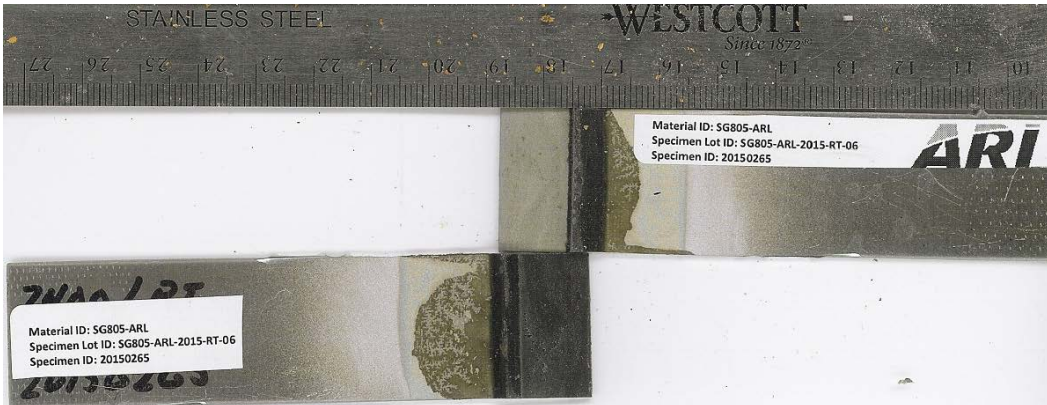
Fig. B-12 Failure surfaces for single-lap-joint with Bonderite M-NT 7400 surface pretreatment. MSAT ID = 20150265, substrate = 2024 T3 aluminum, and sample conditioning = RT. Mode-of-failure = adhesive/ MM.
