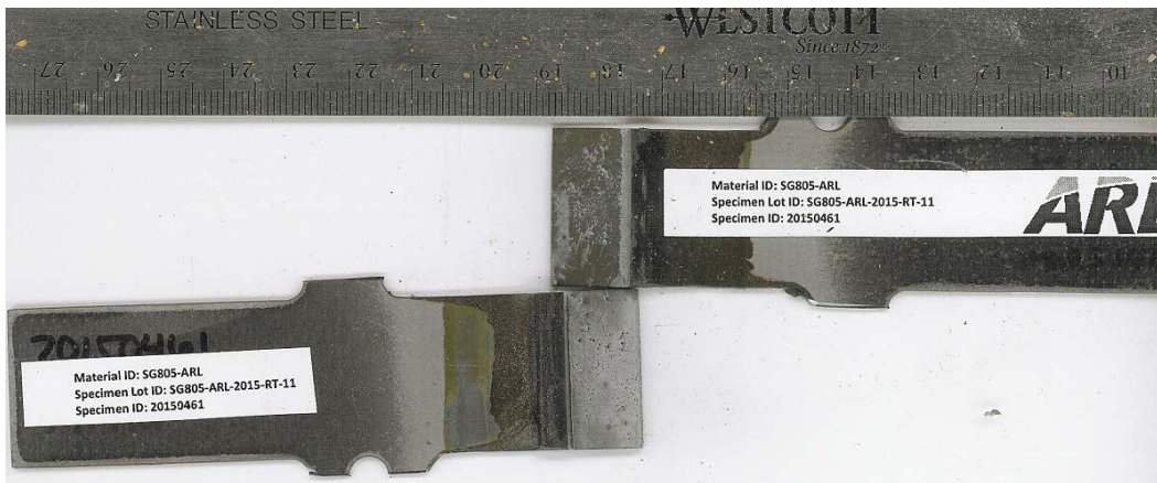
Fig. B-42 Failure surfaces for single-lap-joint with Bonderite M-NT 5700 surface pretreatment. MSAT ID = 20150461, substrate = 1010 steel, and sample conditioning = RT. Mode-of-failure = MM.
