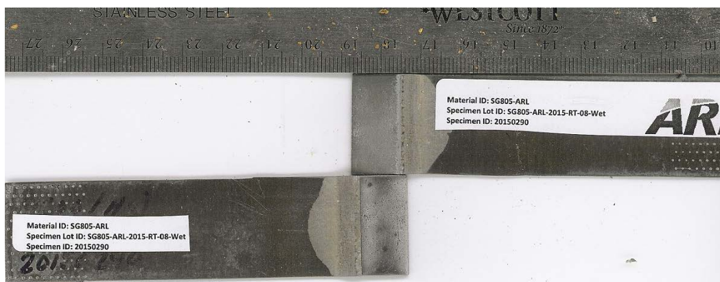
Fig. B-32 Failure surfaces for single-lap-joint with ZIRCOBOND 4200 surface pretreatment. MSAT ID = 20150290, substrate = 2024 T3 aluminum, and sample conditioning = H/W. Mode-of-failure = MM.
