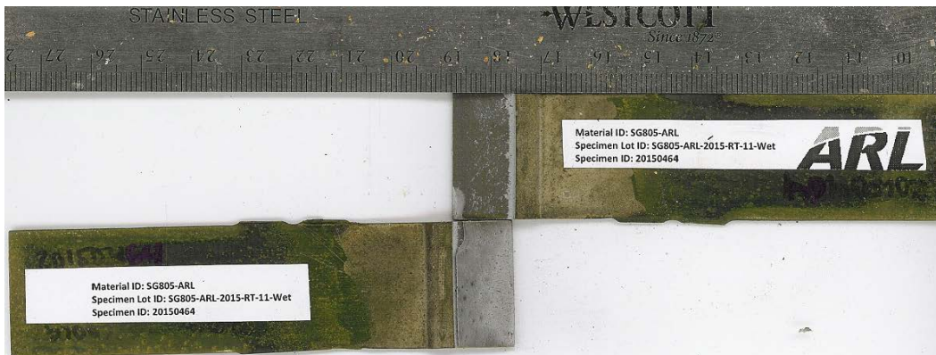
Fig. B-54 Failure surfaces for single-lap-joint with Bonderite M-NT 5700 surface pretreatment. MSAT ID = 20150464, substrate = 1010 steel, and sample conditioning = H/W. Mode-of-failure = MM.
