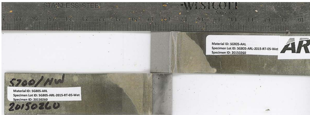
Fig. B-26 Failure surfaces for single-lap-joint with Bonderite M-NT 5700 surface pretreatment. MSAT ID = 20150260, substrate = 2024 T3 aluminum, and sample conditioning = H/W. Mode-of-failure = adhesive/ MM.
