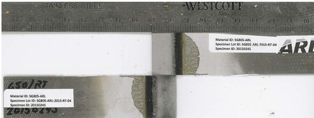
Fig. B-8 Failure surfaces for single-lap-joint with SurTec 650 surface pretreatment. MSAT ID = 20150245, substrate = 2024 T3 aluminum, and sample conditioning = RT. Mode-of-failure = MM.
