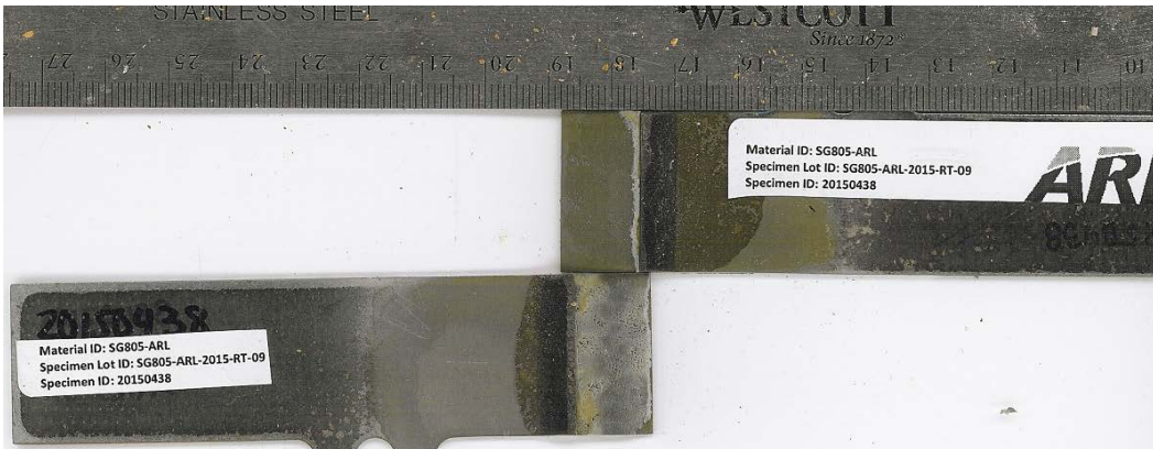
Fig. B-38 Failure surfaces for single-lap-joint with AC-131 BB surface pretreatment. MSAT ID = 20150438, substrate = 1010 steel, sample conditioning = RT. Mode-of-failure = MM.
