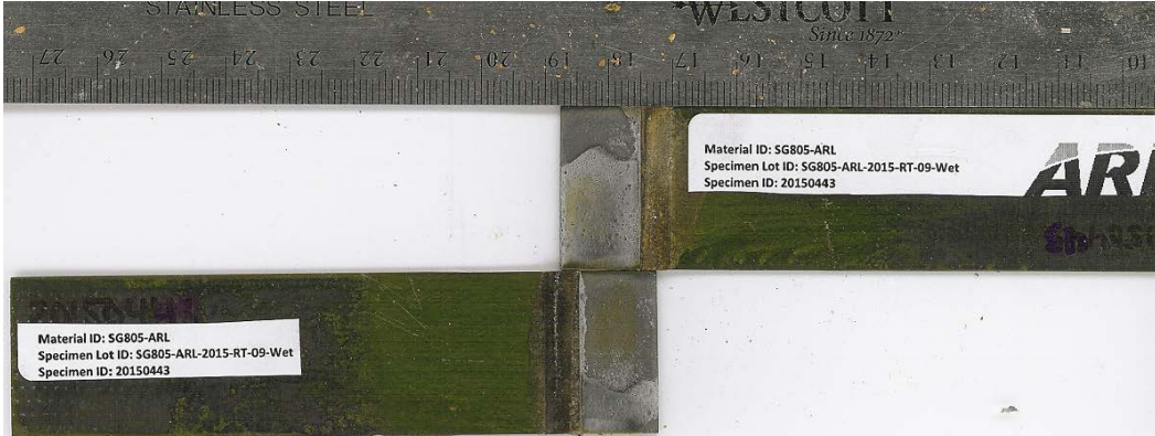
Fig. B-50 Failure surfaces for single-lap-joint with AC-131 BB surface pretreatment. MSAT ID = 20150443, substrate = 1010 steel, and sample conditioning = H/W. Mode-of-failure = MM.
