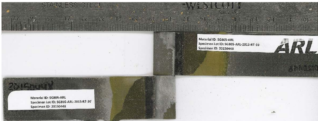
Fig. B-40 Failure surfaces for single-lap-joint with SurTec 650 surface pretreatment. MSAT ID = 20150448, substrate = 1010 steel, and sample conditioning = RT. Mode-of-failure = MM.
