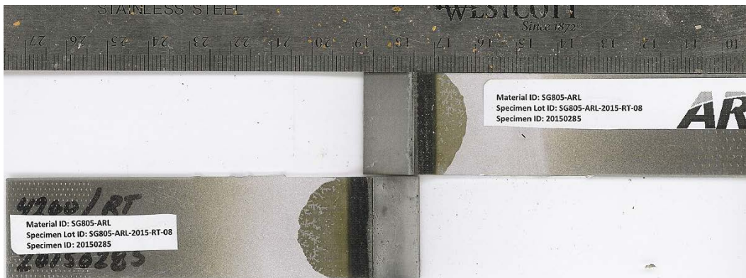
Fig. B-16 Failure surfaces for single-lap-joint with ZIRCOBOND 4200 surface pretreatment. MSAT ID = 20150285, substrate = 2024 T3 aluminum, and sample conditioning = RT. Mode-of-failure = MM.
