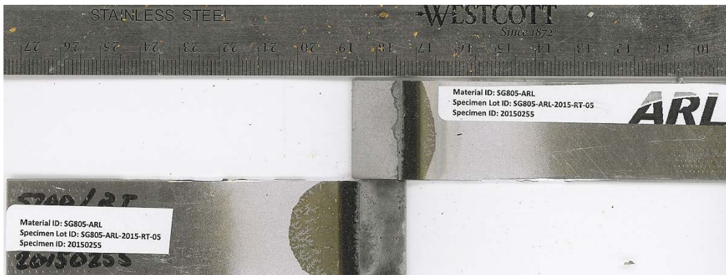
Fig. B-10 Failure surfaces for single-lap-joint with Bonderite M-NT 5700 surface pretreatment. MSAT ID = 20150255, substrate = 2024 T3 aluminum, and sample conditioning = RT. Mode-of-failure = adhesive/ MM.
