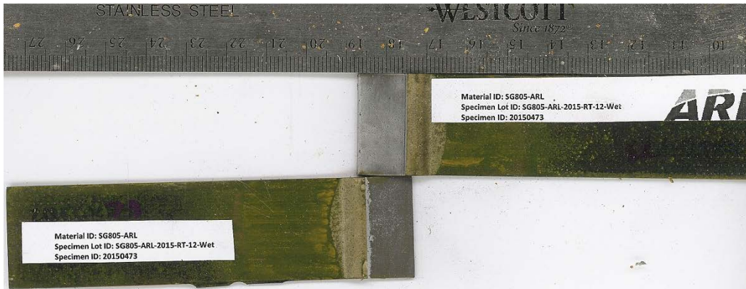
Fig. B-56 Failure surfaces for single-lap-joint with Bonderite M-NT 7400 surface pretreatment. MSAT ID = 20150473, substrate = 1010 steel, and sample conditioning = H/W. Mode-of-failure = MM.
