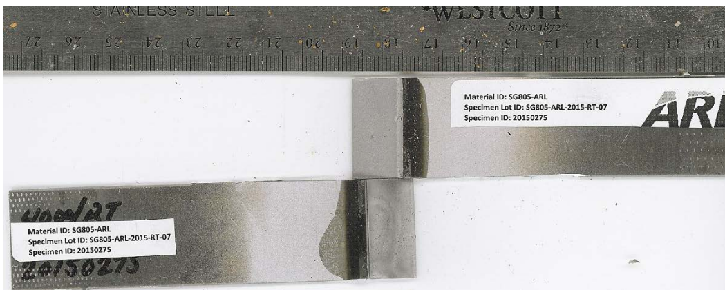
Fig. B-14 Failure surfaces for single-lap-joint with XBOND 4000DM-DR surface pretreatment. MSAT ID = 20150275, substrate = 2024 T3 aluminum, and sample conditioning = RT. Mode-of-failure = adhesive/ MM.
