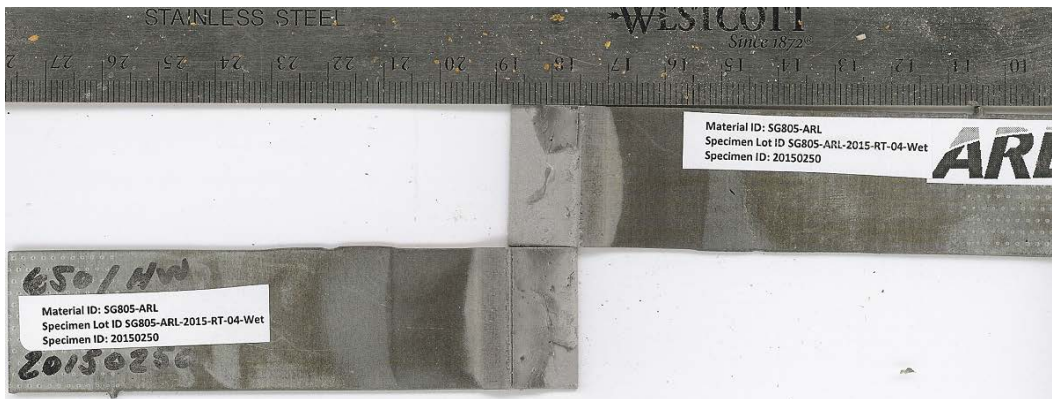
Fig. B-24 Failure surfaces for single-lap-joint with SurTec 650 surface pretreatment. MSAT ID = 20150250, substrate = 2024 T3 aluminum, and sample conditioning = H/W. Mode-of-failure = MM.
