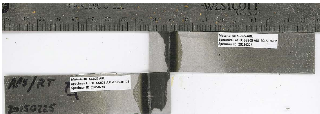
Fig. B-4 Failure surfaces for single-lap-joint with 3-aminopropyltrimethoxysilane surface pretreatment. MSAT ID = 20150225, substrate = 2024 T3 aluminum, and sample conditioning = RT. Mode-of-failure = adhesive.
