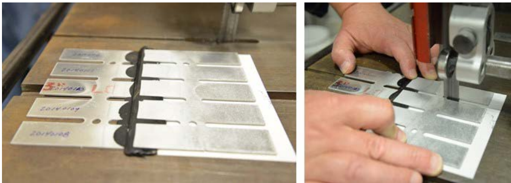
Fig. 22 “Intact” bonded single-lap-joint panel showing adhesive fillets, side overflow, and the cardboard shim (left) and each individual single-lap-joint coupon specimen being separated from the panel using a band saw (right)
