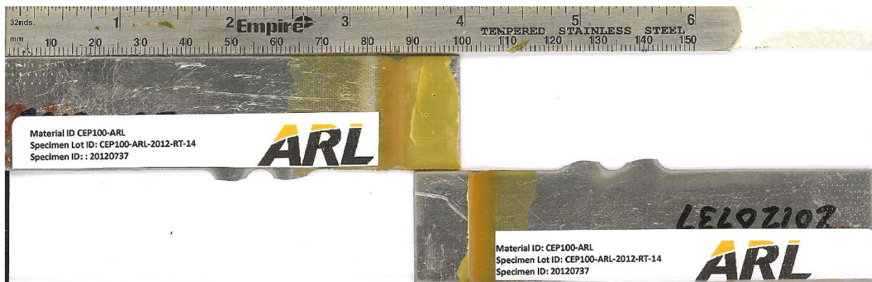
Fig. 32 Representative scanned failure surfaces showing sample ID information embedded within the image (ruler is included for quantitative dimensional scaling)
