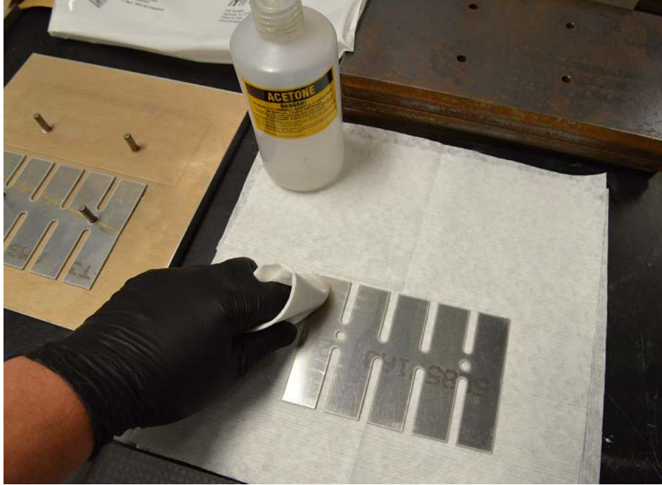
Fig. 2 Surface treating the lap-joint coupon panel using the acetone solvent wipe surface preparation method
