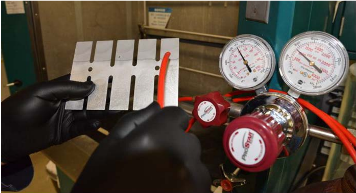
Fig. 5 View showing the typical gas spray cleaning process used to remove residual surface grit medium after the grit-blasting process from tab bonding surfaces
