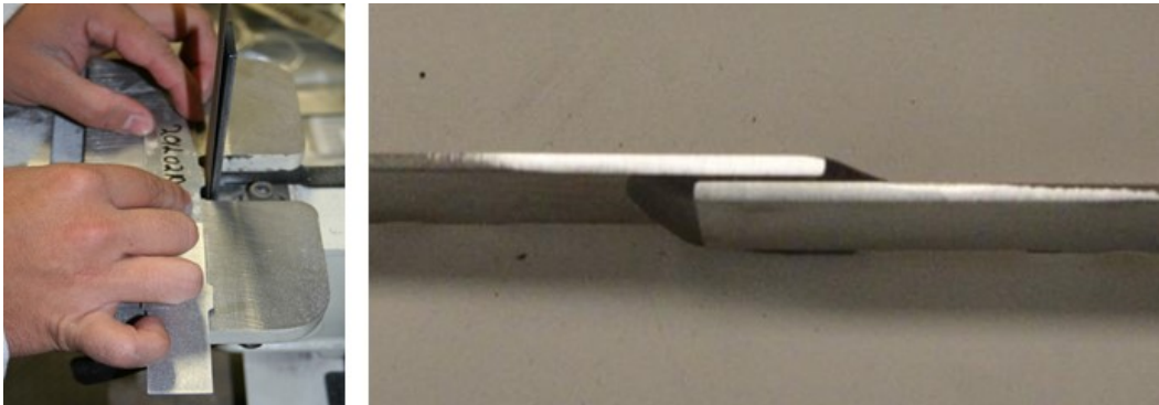
Fig. 23 Finishing preparation of a single-lap-joint coupon test specimen using a belt sander (left) and a side view of the test specimen after removing the excess adhesive (right)
