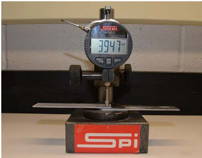
Fig. 24 Perform the single-lap-joint bondline thickness measurements using a calibrated micrometer
