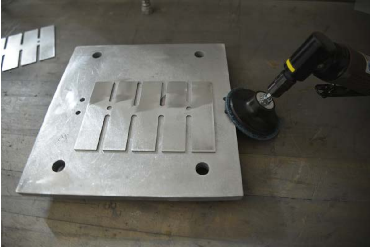
Fig. 4 Heavy surface oxidation may be removed prior to grit blasting using an abrasion pad (Scotch-Brite 048011-65530 A VFN, or equivalent)
