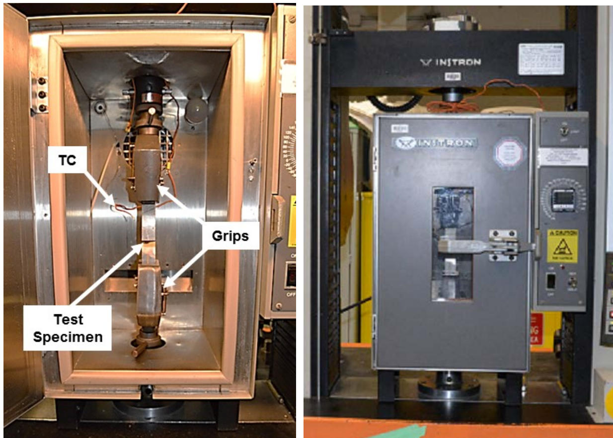
Fig. 27 Samples undergoing elevated temperature testing at 71 °C, \pm 3 °C (160 °F, \pm 5 °F), with the chamber door opened (left) and closed (right)
