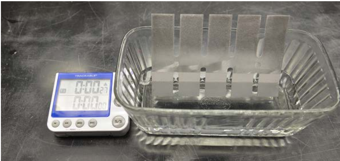
Fig. 6 Immersion of grit-blasted primed aluminum single-lap-joint coupon panel tabs submerged in the GPS silane coupling agent solution bath for 90 s by the clock
