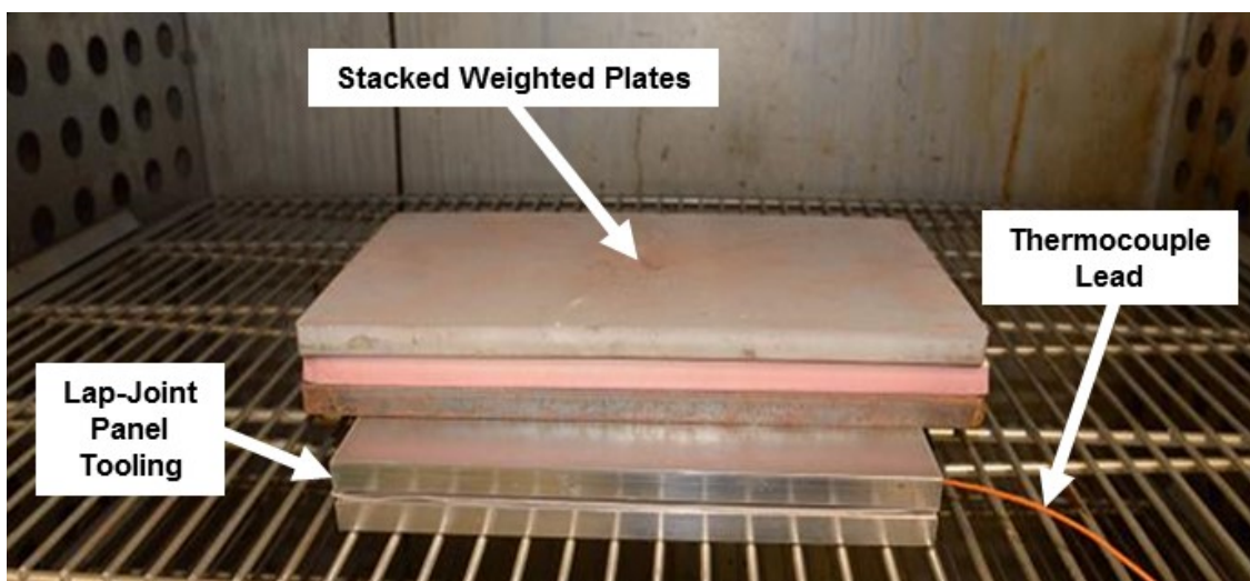
Fig. 20 Representative example of the plate-loaded single-lap-joint tooling fixture undergoing oven cure at elevated temperature
